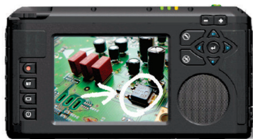
Two-way annotation capabilities enable users to highlight areas of a still image on the device and stream them to the expert at the PC — or vice versa.
